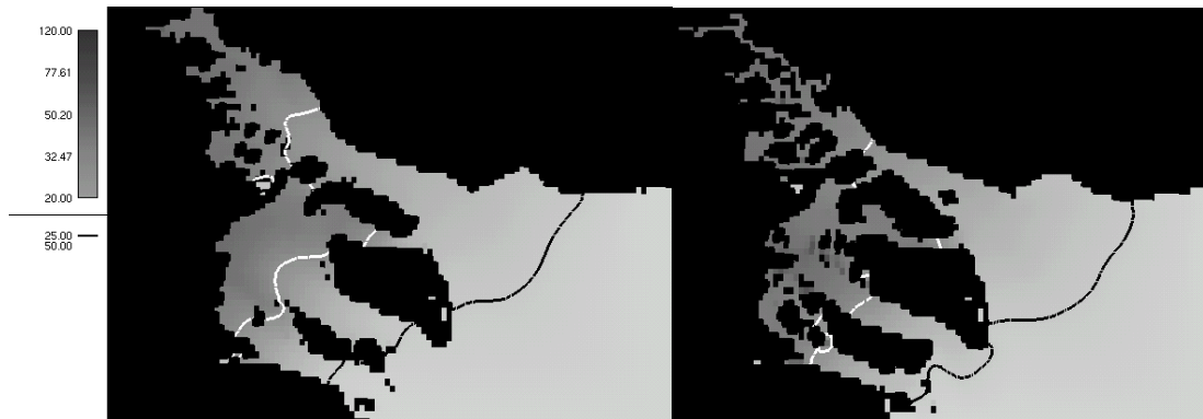
Figure 15 Cohesive sediments concentration ( \text{mg l}^{-1} ) in the water column during flood (left) and ebb tide (right).
